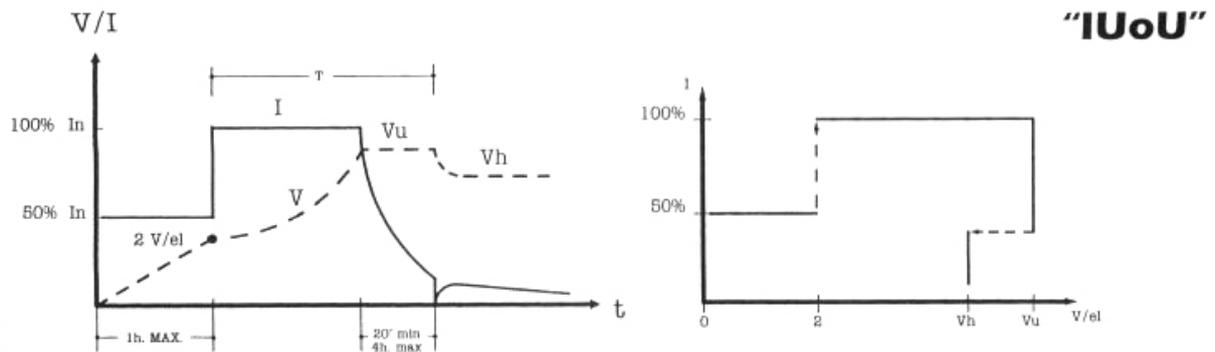
$T = 12 + 14 \text{ h} \quad I_n = \frac{C_B (\text{Ah})}{6}$
